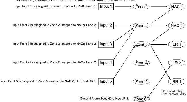
The following example shows how inputs drive zones and zones drive outputs.
