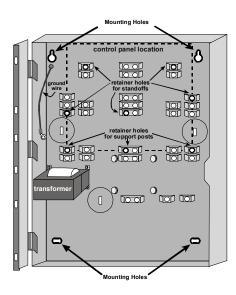
Figure 3: Enclosure Installation
