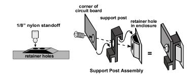
Figure 4: Standoff and Support Post Installation
