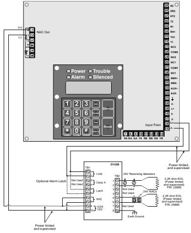
Figure 13: Wiring the D132B
