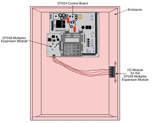
Figure 12: D7039 Mounting Location
