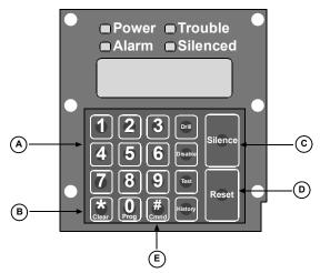
Figure 11: Keys Essential to Alpha Programming
