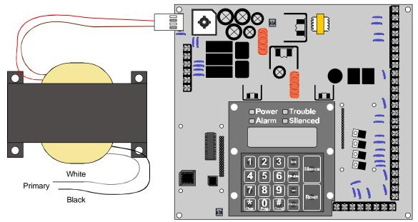
Figure 6: Connecting the Transformer to the D7024 Control Board
